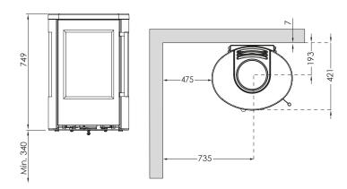
TT23RGW is designed for mounting on a non-flammable wall. If the floor covering is flammable, the stove must be mounted at least 340 mm above the floor. Talk to your dealer and/or chimney sweep about the best fireproof mounting solution.
