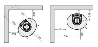
In order to avoid discolouration of painted and treated surfaces, TermaTech recommends the same distance from flammable materials as for non-flammable materials. This distance increases the convection itself around the stove and also eases cleaning. All distances relate solely to the distance of the stove from flammable materials. No account has been taken of national requirements for the use of stove flues or their distance from flammable materials.
