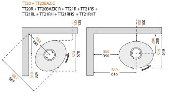
In order to avoid discolouration of painted and treated surfaces, TermaTech recommends the same distance from flammable materials as for non-flammable materials. This distance increases the convection itself around the stove and also eases cleaning. All distances relate solely to the distance of the stove from flammable materials. No account has been taken of national requirements for the use of stove flues or their distance from flammable materials.
